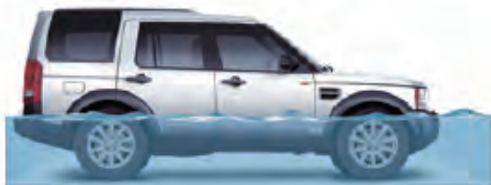
MAXIMUM WADING DEPTH 700 mm (27.6 in.)
