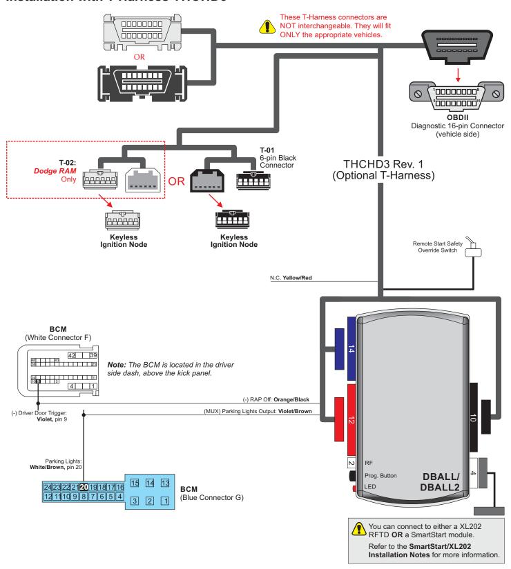
With the exception of the OBDII Diagnostic connector, all adapters are displayed from the wire side (unless specified otherwise).
