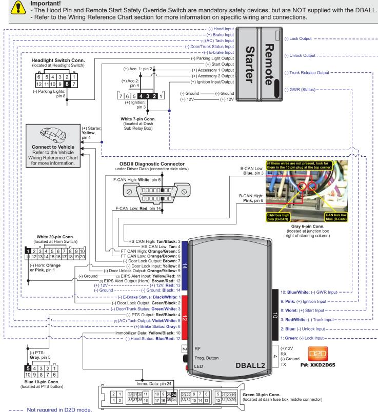
[1] Tach wire is an optional connection required on some remote starters, which do not support a tach signal in D2D.
