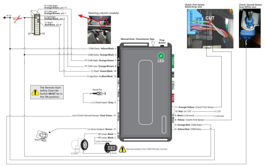
A While there are 2 possible versions of wiring harnesses, this diagram uses the CURRENT harness. Refer to the Wiring connections section for more information.
