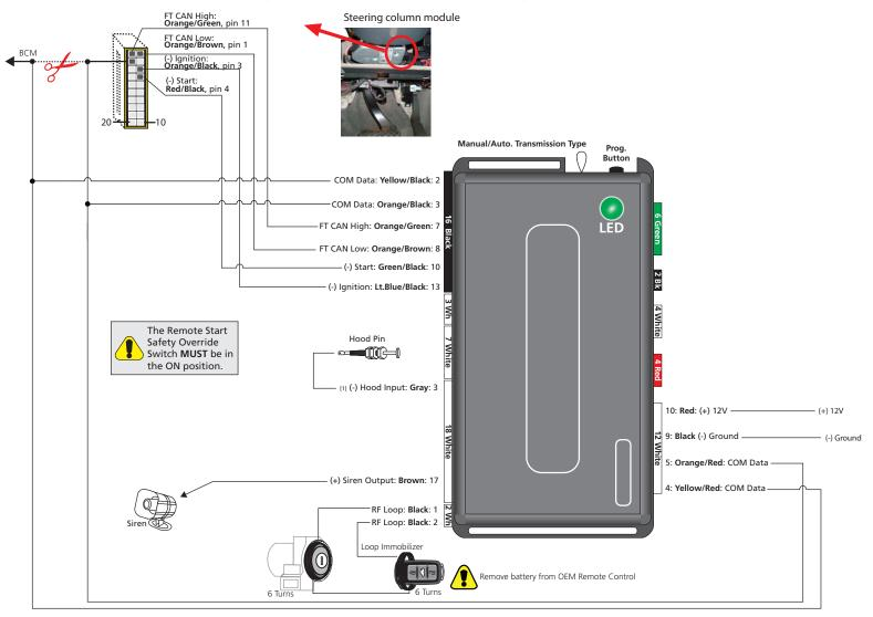
🗛 While there are 2 possible versions of wiring harnesses, this diagram uses the CURRENT harness. Refer to the Wiring connections section for more information.
