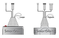
**DO NOT** connect the SmartStart 2-pin power harness when using the Directed Digital Solutions. Power and ground will be provided by the D2D connector on main module. Refer to the SmartStart documentation for further details.
