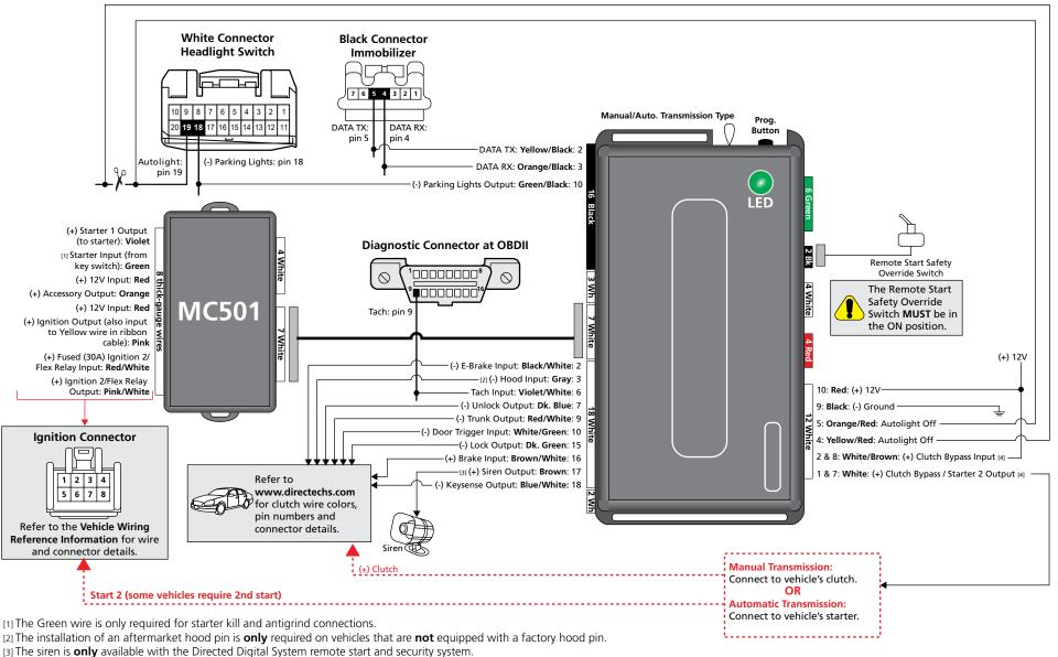
[4] Reprogramming the default feature to starter is required for the clutch bypass.
