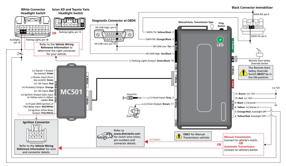
[1] The Green wire is only required for starter kill and antigrind connections.
