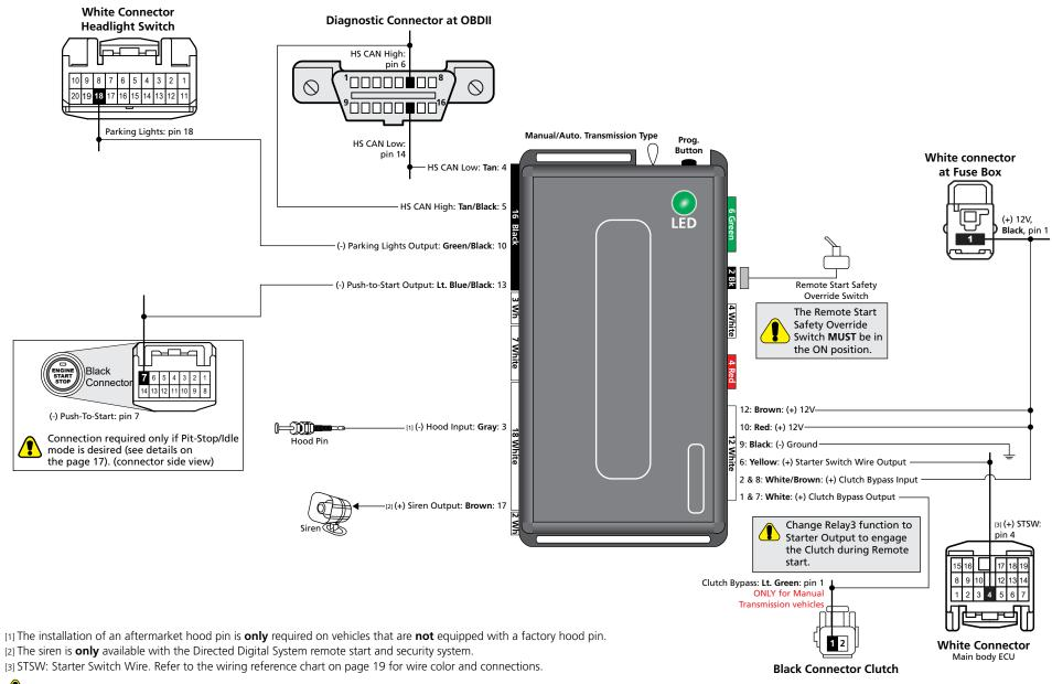
🕐 With the exception of the OBDII diagnostic connector, all adapters are displayed from the wire side (unless specified otherwise).
