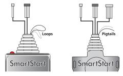
DO NOT connect the SmartStart 2-pin power harness when using the DS4+. Power and ground will be provided by the D2D connector on main module. Refer to the SmartStart documentation for further details.
