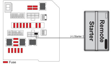
Starter Wire Voltage Test (Multimeter) Automatic & Manual Transmission
