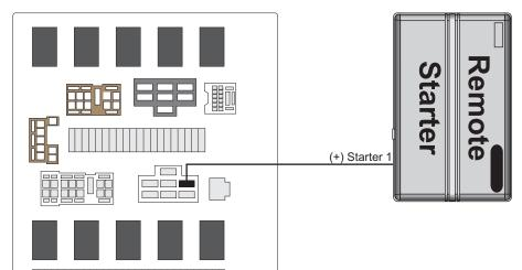
Starter Wire Voltage Test (Multimeter) Automatic & Manual Transmission
