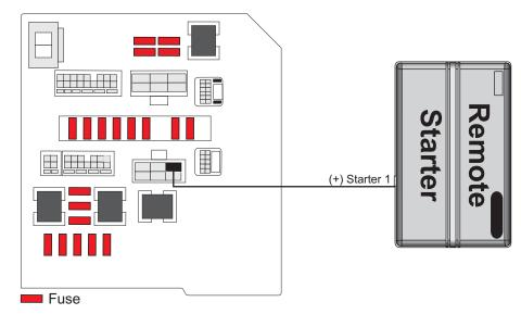
Starter Wire Voltage Test (Multimeter) Automatic & Manual Transmission
